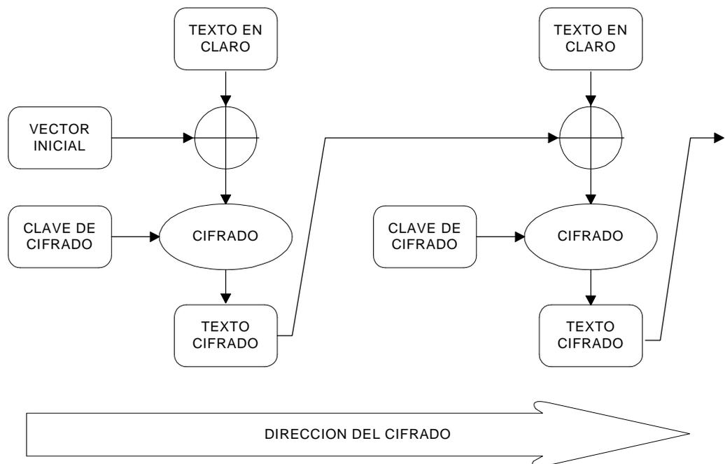
$$c_i = C_k(m_i \oplus c_{i-1}) \quad \text{con } c_o = C_k(V_i)$$
